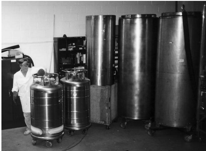
Stainless steel high-vacuum cryostats may hold one cryonaut or as many as four. Liquid nitrogen fills up the cryostats.
